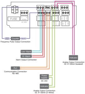
Wiring connection on sensor to converter
