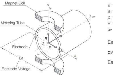
E = Electrode Voltage B = Magnetic Induction D = Electrode Distance V = Average Flow Velocity qv = Volume Flowrate  $Ea \sim B \cdot D \cdot v$
