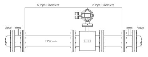
Upstream and Downstream straight pipe diameter
