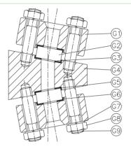
G1. Cover plate G2. Gauge glass G3. Mica gasket G4. Gauge body
